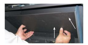
6) Remove the two side brackets and screws (set aside) - then remove the side panels by tilting the top in and lifting them out.
